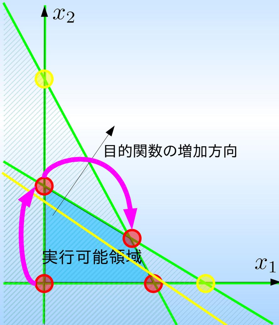
$$\begin{aligned} & \text{maximize} \\ & 600x_1 + 500x_2 \\ & \text{subject to} \\ & 3x_1 + x_2 \leq 45 \times 10^3 \\ & x_1 + 2x_2 \leq 40 \times 10^3 \\ & x_1, x_2 \geq 0 \end{aligned}$$
