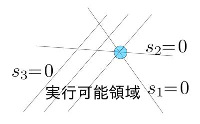
$$\begin{array}{c} \text{minimize} \\ z = x_1 + 2x_2 \\ \text{subject to} \\ x_1 + x_2 - s_1 = 4 & \textcircled{1} \\ -x_1 + 2x_2 - s_2 = 2 & \textcircled{2} \\ -x_2 - s_3 = -3 & \textcircled{3} \\ x_1, x_2 \geq 0 \end{array}$$
