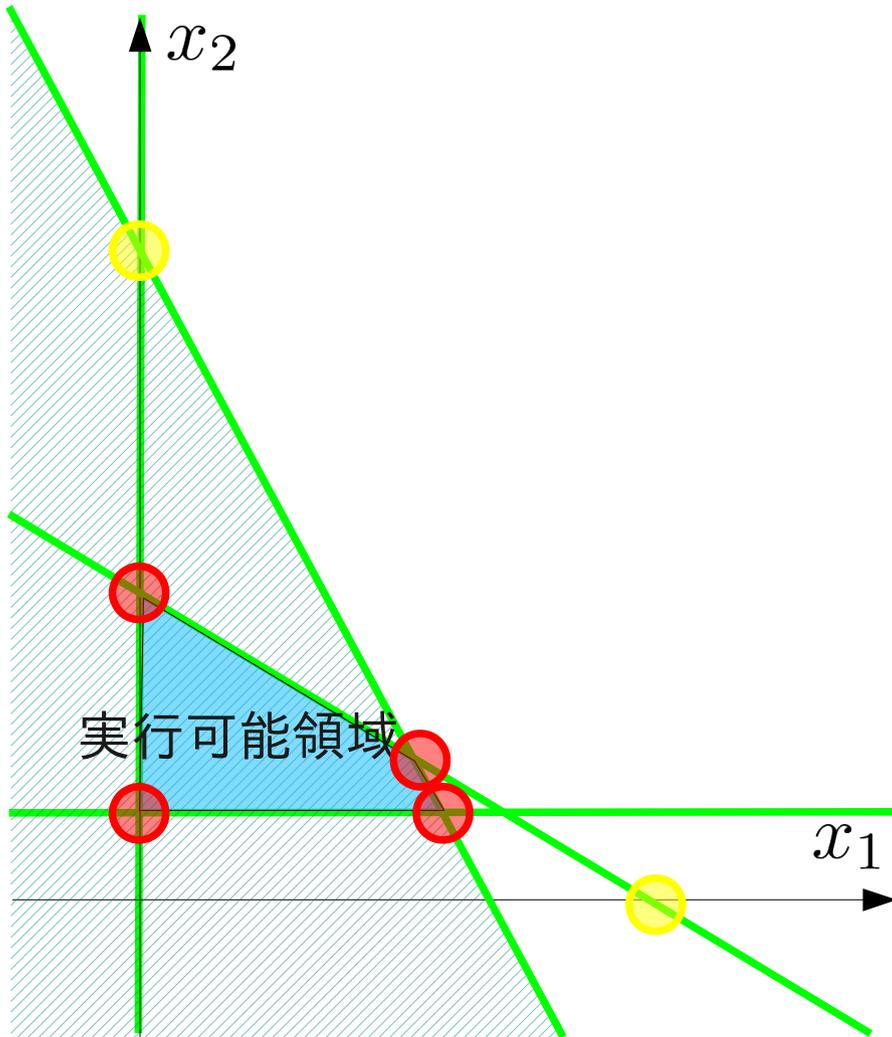
$$\begin{aligned} & \text{maximize} \\ & 600x_1 + 500x_2 \\ & \text{subject to} \\ & 3x_1 + x_2 \leq 45 \times 10^3 \\ & x_1 + 2x_2 \leq 40 \times 10^3 \\ & x_2 \geq 10 \times 10^3 \\ & x_1, x_2 \geq 0 \end{aligned}$$
