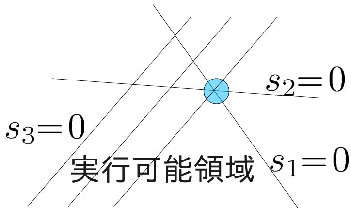
$$\begin{aligned} & \text{minimize} \\ & z = x_1 + 2x_2 \\ & \text{subject to} \\ & x_1 + x_2 - s_1 = 4 \quad ① \\ & -x_1 + 2x_2 - s_2 = 2 \quad ② \\ & -x_2 - s_3 = -3 \quad ③ \\ & x_1, x_2 \geq 0 \end{aligned}$$
