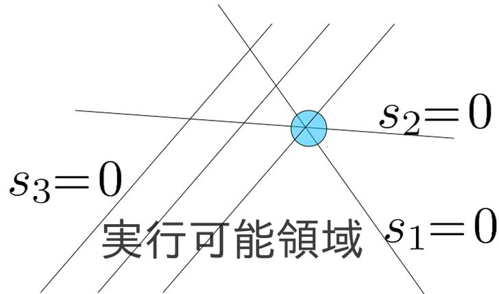
$$\begin{aligned} & \text{minimize} \\ & z = x_1 + 2x_2 \\ & \text{subject to} \\ & x_1 + x_2 - s_1 = 4 \quad \textcircled{1} \\ & -x_1 + 2x_2 - s_2 = 2 \quad \textcircled{2} \\ & -x_2 - s_3 = -3 \quad \textcircled{3} \\ & x_1, x_2 \geq 0 \end{aligned}$$
